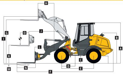
324L STANDARD-LINKAGE / HIGH-LIFT-LINKAGE LOADERS WITH QUIK-TATCH COUPLER AND FORK
